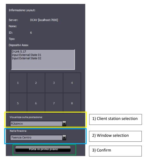
The client will be selected using a combo-box containing the list of client stations logged onto the server. As a consequence, it will be possible to send the request to only one client at a time.
