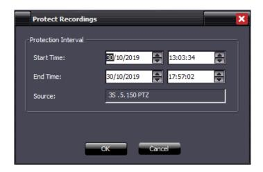
Once you have pressed "ok" the protection procedure will be started and this will result in a final message highlighting the initial and final instant of the protected recording.
