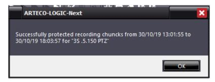
The protection of a portion of the recording will be at the level of the single ".eye" file. This means that, if you select a recording portion for protection, the actual protection will be a larger section (or at most equal), since it depends on the size of the file or files that belong to the interval selected by the user.
