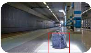
**AE-Lost:** it is the video analytic module which allows to detect abandoned and/or removed objects (for instance objects abandoned in public areas such as airports, train stations or metro stations). AE-Lost can be installed both indoor and outdoor, combined with both thermal and traditional cameras.
