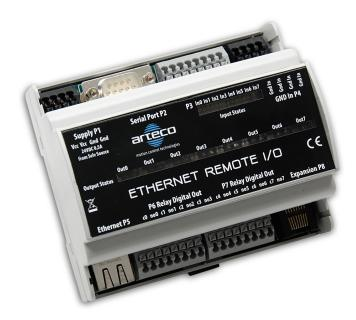
This is the new ethernetl remote I/O module from Arteco, suitable for both industrial and home applications.
